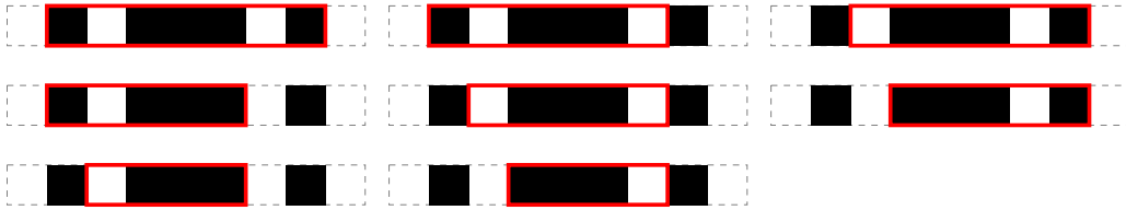
Figure 4.6: Unique divisions that include the center of the finder pattern based only on the edge ratio information.
