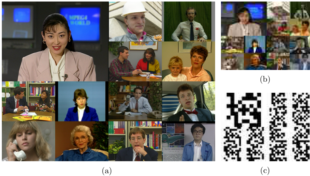
Figure 4.3: A 13-participant conference as (a) 1440 \times 1080 pixel high quality version, (b) highly compressed 128 \times 96 pixel low quality mobile version, (c) highly compressed 128 \times 96 pixel low quality mobile version with encoded data for automatic layout determination.
