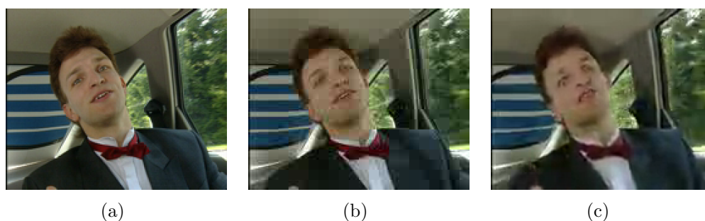
Figure 2.8: Blocking and blurring artifacts created by low bitrate encoding of (a) the original image by (b) H.263 encoder and (c) H.264 encoder.
