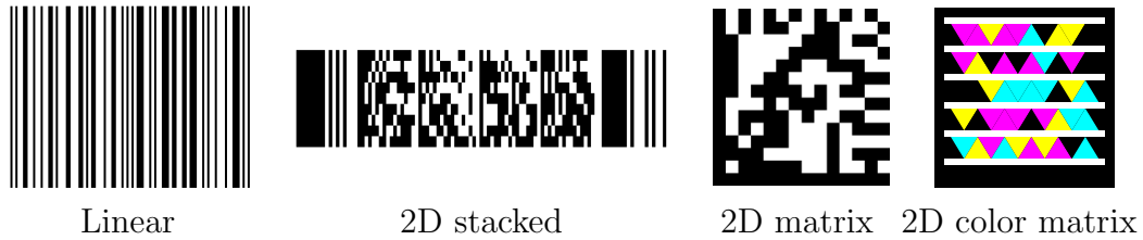
Figure 3.2: Evolution of barcodes from one-dimensional linear barcodes to color coded two-dimensional barcodes.
